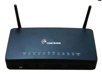
The VG-8061u is an advanced Gigabit Ethernet gateway with 1 Gigabit Ethernet WAN port, 4 Gigabit Ethernet LAN ports, 2 FXS ports, and Wi-Fi. The Wi-Fi not only provides an 802.11n 2T2R 2.4GHz Band which is backward compatible with 802.11b/g but also supports high performance 802.11ac with 3T3R design at 5GHz band.
